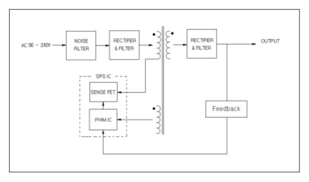
Circuit topology : flyback(CS15), forward(CS30,CS50) Switching frequency : 100KHz(fixed)
